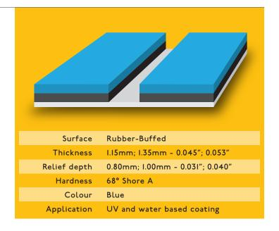
Since the Blanket's structure has no fabric, any problems related to "fabric impression" are completely eliminated; therefore it also limits the gauge reduction, improves smash resistance and prevents coating and cleaning agents from penetrating into the blanket. After cutting, the blanket shows no fibres on the cut edge.
